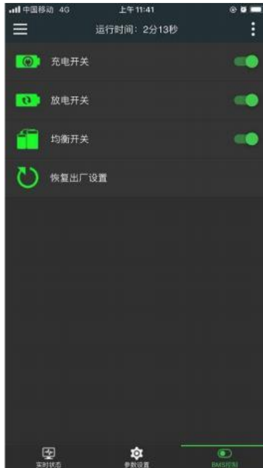
Figure 38 BMS control page
