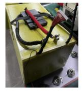
8. Put the battery into the box and fix the cache cotton on the battery
